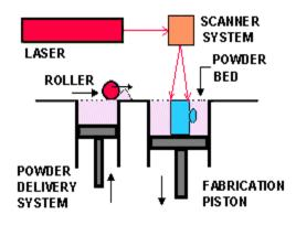
After the object is fully formed, the piston is raised to elevate it. Excess powder is simply brushed away and final manual finishing may be carried out. No supports are required with this method since overhangs and the solid powder bed supports undercuts.
